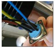
Install the connector from the bottom side of the gas damper bracket.
